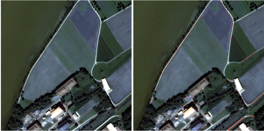
Figure 13.11: Result of applying the road extraction by steps pipeline to a fusionned Quickbird image. From left to right : original image, extracted road with their likelihood values.
