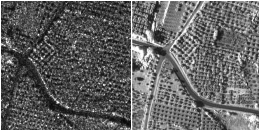
Figure 8.7: A SAR image (fixed image) and an aerial photograph (moving image) are provided as input to the registration method.
