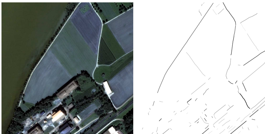
Figure 13.9: Result of applying the otb::RoadExtractionFilter to a fusionned Quickbird image. From left to right : original image, extracted road with their likelihood values (color are inverted for display).
