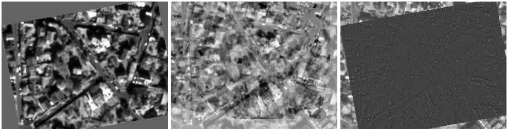
Figure 8.12: Resampled moving image (left). Differences between the fixed and moving images, before (center) and after (right) registration with the CenteredRigid2D transform.
