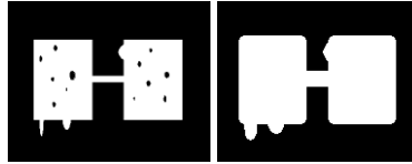
Figure 19.9: The effects of morphological operations on a binary image using a circular structuring element of size 4. Left: original image. Right: dilation.
