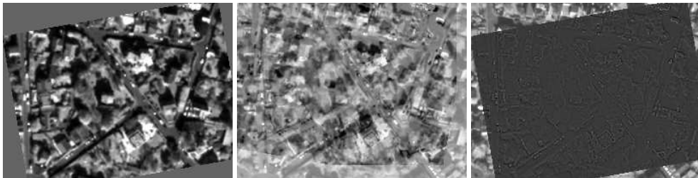
Figure 8.14: The resampled moving image (left), and the difference between the fixed and moving images before (center) and after (right) registration with the AffineTransform transform.
