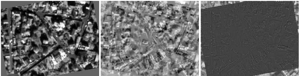
Figure 8.10: Resampled moving image (left). Differences between the fixed and moving images, before (center) and after (right) registration using the CenteredRigid2D transform.
