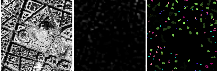
Figure 15.8: Morphological pyramid segmentation. From left to right: original image, image of bright details and result of the segmentation.
