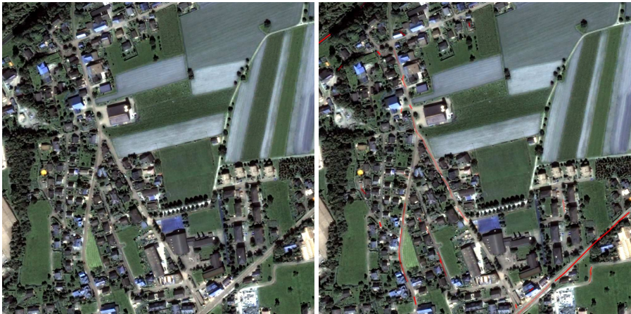
Figure 13.12: Result of applying the road extraction by steps pipeline to a fusionned Quickbird image. From left to right : original image, extracted road with their likelihood values.
