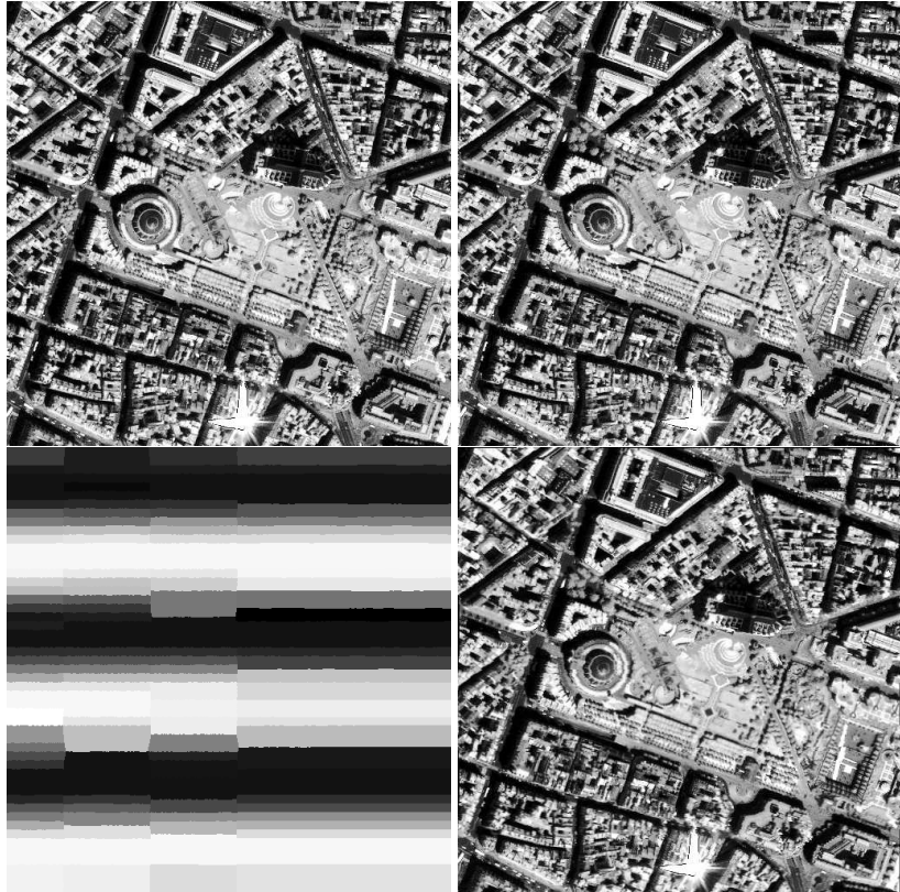
Figure 9.2: From left to right and top to bottom: fixed input image, moving image with a sinusoid deformation, estimated deformation field in the horizontal direction, resampled moving image.
